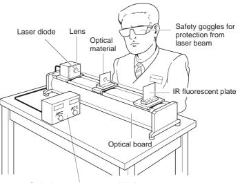
Optical power output control device Temperature control device
